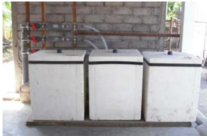
Insulated drums for comparative laminar flow compost research
