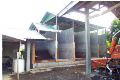
4 meter high laminar flow boxes, simulating the large scale facility
